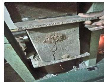
Visible cracks during compression
