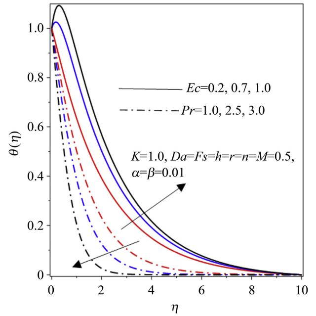
**Figure 7** Effect of  $Ec$  and  $Pr$  on heat field.
