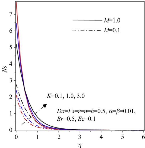
Figure 8 Entropy field for rise in  $M$  and  $K$ .
