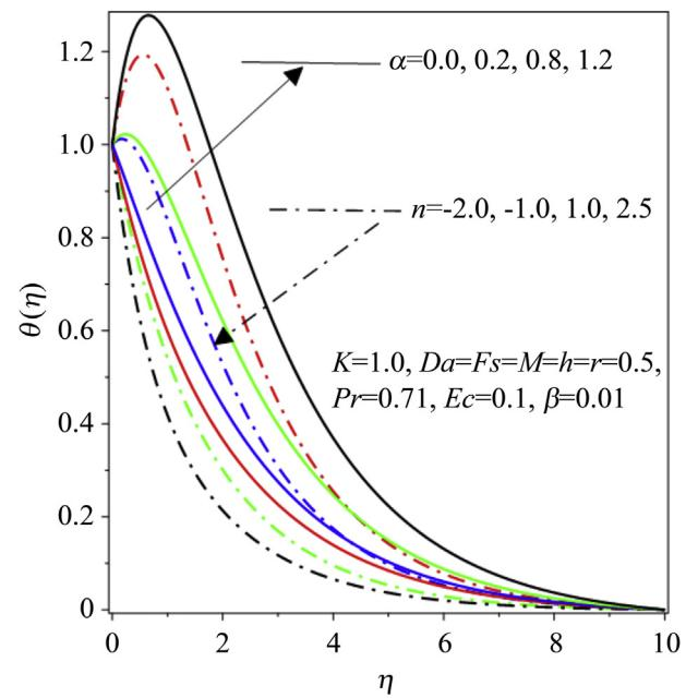
**Figure 6** Heat field for rise in  $\alpha$  and  $n$ .
