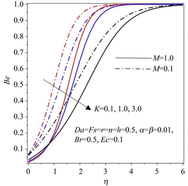
Figure 10 Bejan field for various  $M$  and  $K$ .
