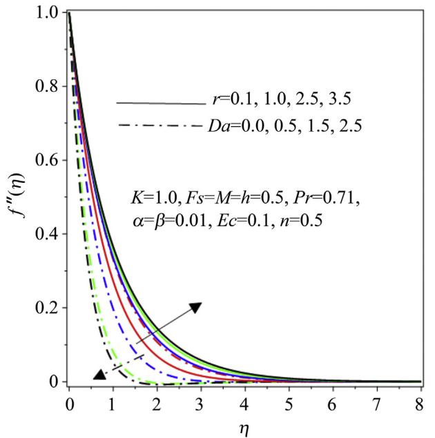
**Figure 3** Velocity field for rising  $r$  and  $Da$ .
