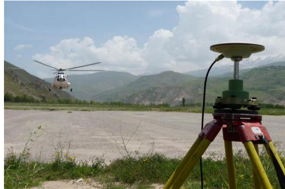
Figure 4: Surveyors setting out Airport facilities Figure 5: DGPS observation at Helicopter landing
