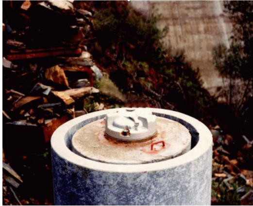
Figure 7: Survey Network station at Monte Novo dam site. Source: (Henriques, Maria João & Casaca, João, 2004)
