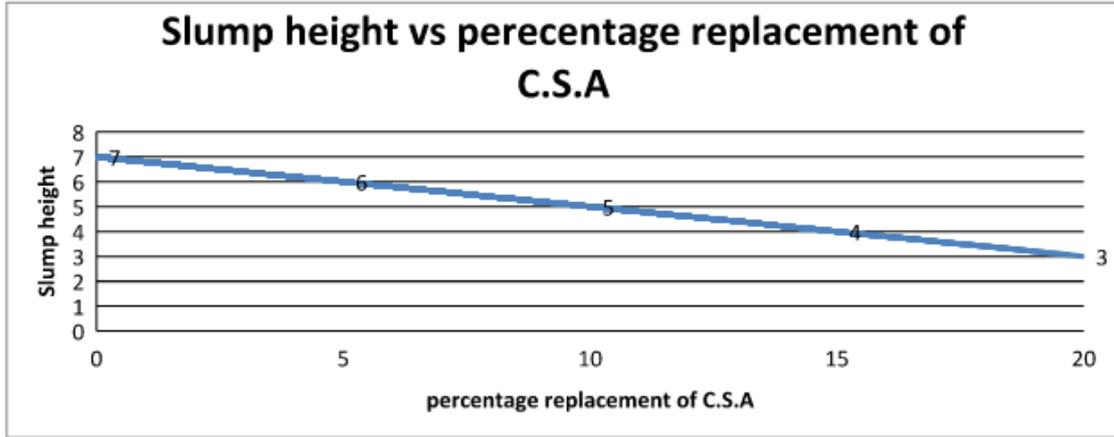
Fig .6: Graph of slump against percentage replacement of CSA in concrete. It was observed that control has slump height of 7mm and decreased to 6mm at 5% replacement of the C.S.A in concrete then later increased to 5mm at 10%, later dropped to 4mm at 15% and finally declined to slump height of 3mm at 20% replacement.
