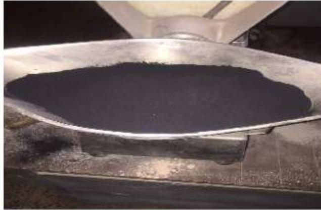
Fig.3: Coconut shell ash
