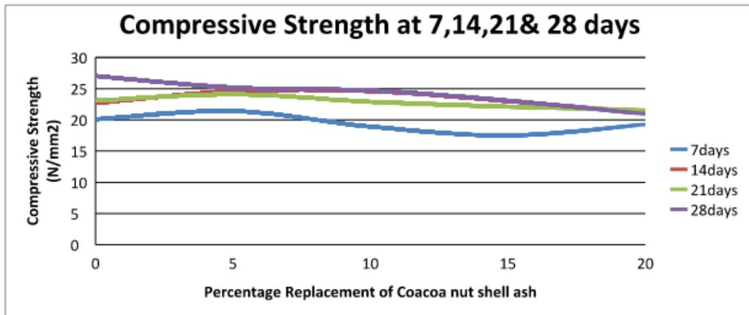
Fig .7: Compressive strength development with the curing days.
