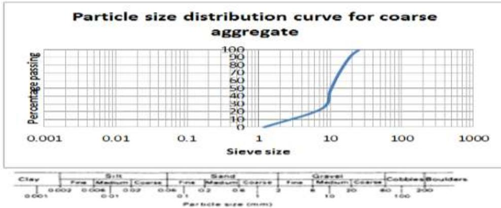
Fig.4: Particle size distribution curve for coarse aggregate (granite).
