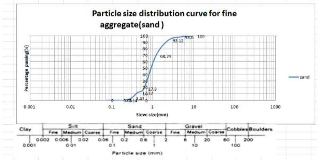
Fig.5: Particle size distribution curve for fine aggregate (sand).
