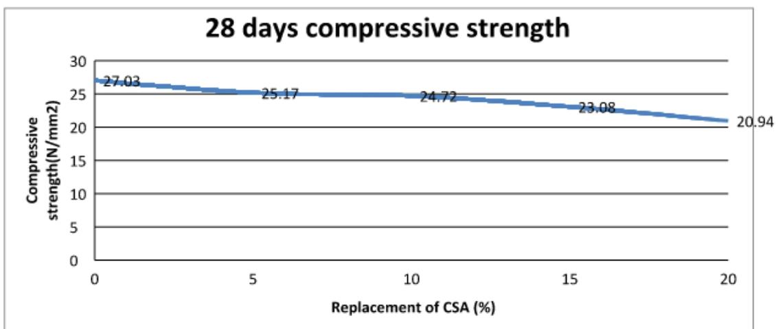
Fig .8: 28 days compressive strength against percentage CSA concrete.
