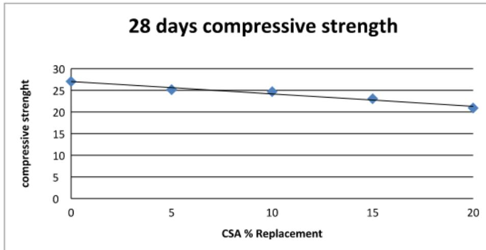
Fig. 9: Regression analysis that show relationship between compressive strength and percentage replacement of CSA
