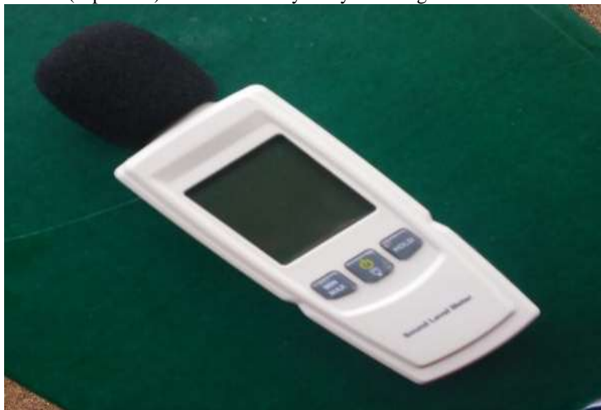
Figure 1-Sound level meter (GB: 2266204, made in China)
