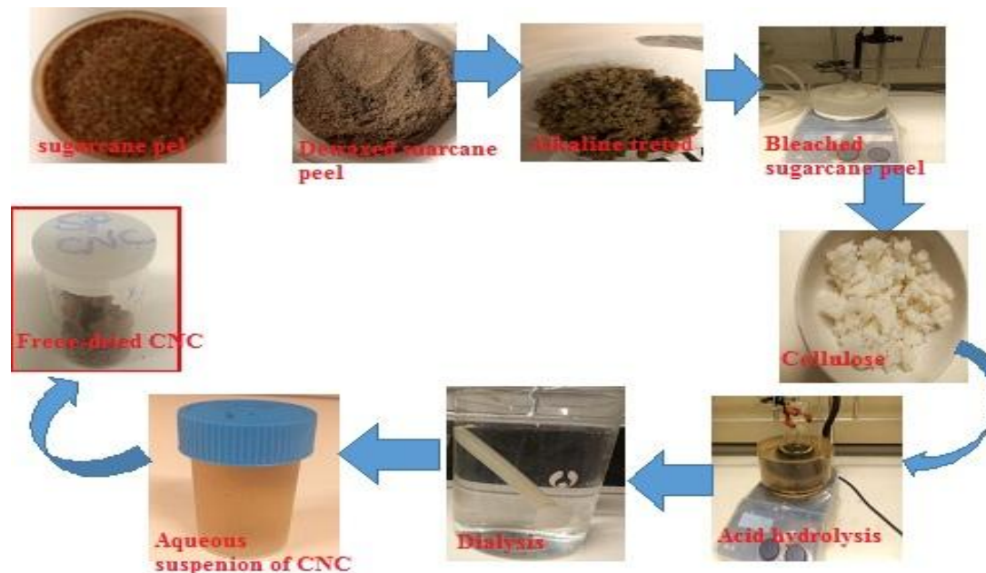
Figure 1: Schematic representation of the preparation of cellulose nanocrystal from sugarcane peel.
