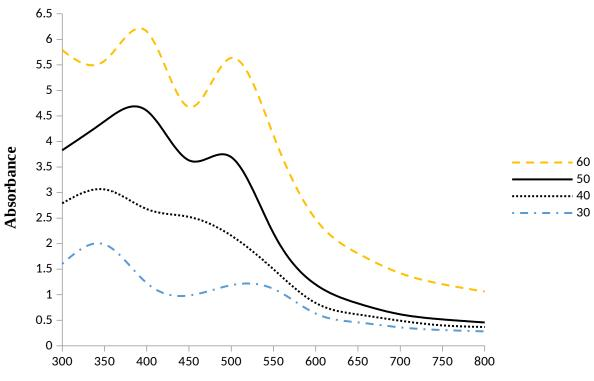
ure 5: The UV-Visible spectrum of synthesised TC-AgNPs at different temperature intervals
