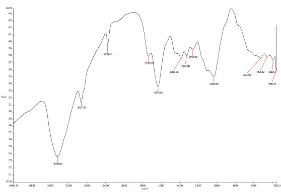
Figure 6: The FTIR spectrum of synthesised TC-AgNPs
