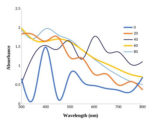
Figure 4: The UV-Visible spectrum of synthesised TC-AgNPs at different time intervals
