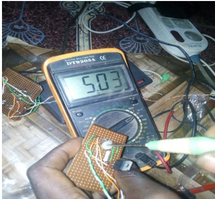
Figure 8: Testing and adjustment of input voltage
