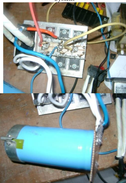
Figure 8 and 9: Power Inverter showing the six IGBTs and the 2,500µF Capacitance Filter used
