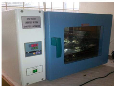
**Figure 4:** Laboratory oven (search tech instrument DHG-9053A)
