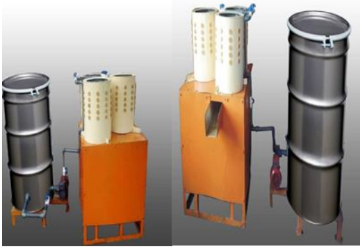
Figure 13. A pictorial view of the fabricated defeathering machine
