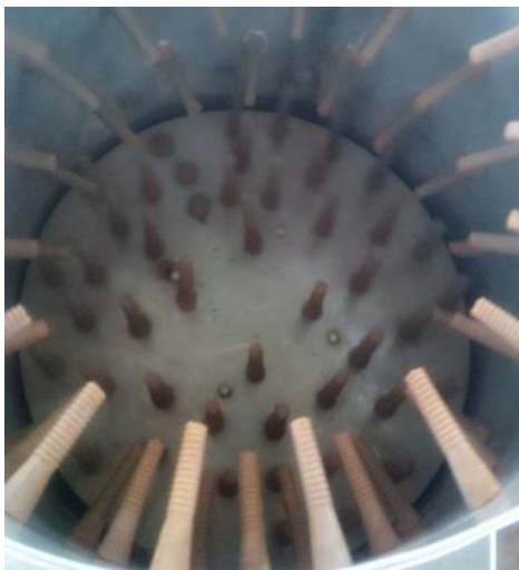
Figure 14. Inner part of the defeathering chamber (rotating plate and rubber pluckers)
