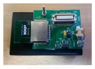
Figure 2.0 Radio module
