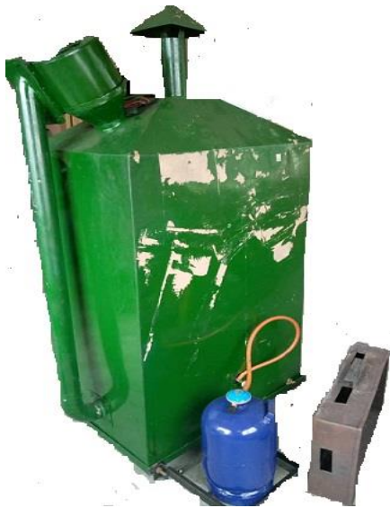
Figure 9. Mechanical dryer showing dual heat sources used for the experiment.
