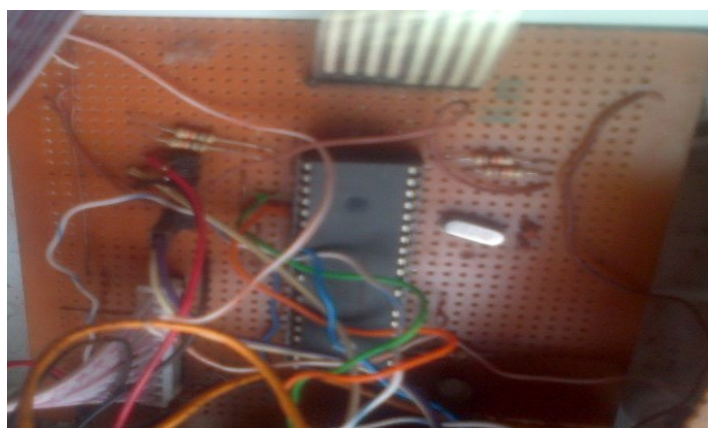
Plate 1: Soldered Components on the Vero board
