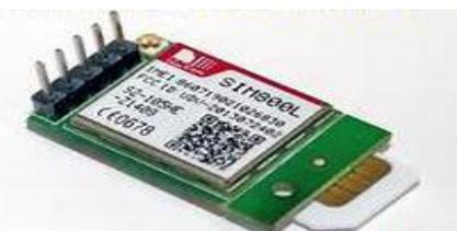
**Fig. 3.4: SIM 800L GPRS Module with SIM card**
