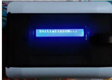
Figure 4.2a: The Gas leakage detector showing Initialization at Power On.
