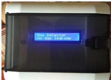
Figure 4.2d: The Gas leakage Detector System with status “no gas leakage detected”
