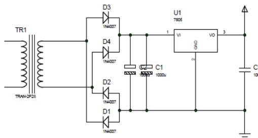
**Figure 3.5: Complete Power Supply Circuit**
