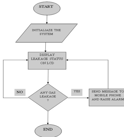
Figure 4.3: Flowchart for Mode of operation of the Constructed Microcontroller Based Combustible Gas leakage Detector System with SMS Notifications and Power Back up.
