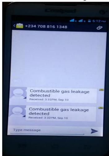
Figure 4.2f: The Mobile phone showing the SMS notification received after leakage Detection.
