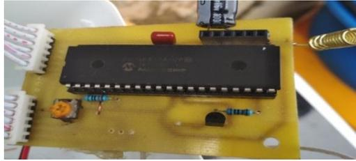
Figure 4.1b: The PCB Showing Microcontroller (16F877A) used and other components.
