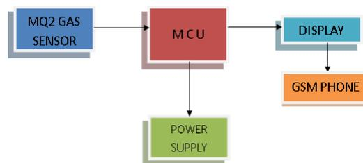
**Figure 3.1:** Block diagram of Microcontroller Based Gas Leakage Detector with Buzzer and SMS Notification System.
