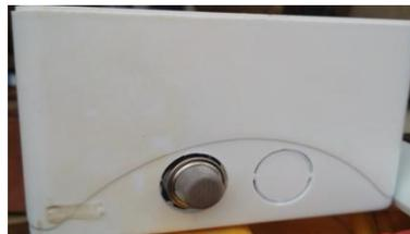
Figure 4.2c: Showing the MQ-2 Gas Sensor embedded with the System
