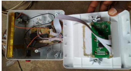
Figure 4.1c: Showing the Circuit Boxing with Built-in Rechargeable Power Back up
