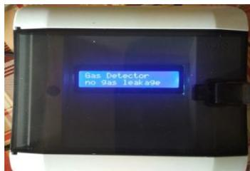
Figure 4.2g: The Gas leakage Detector System with status “no gas leakage detected”.
