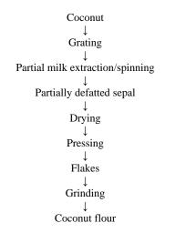
Fig 1(a): Flow chart for the production of coconut flour
