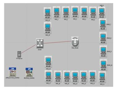
Fig. 2. Modeling of Wireless Local Area Network (WLAN) with 20 Workstations
