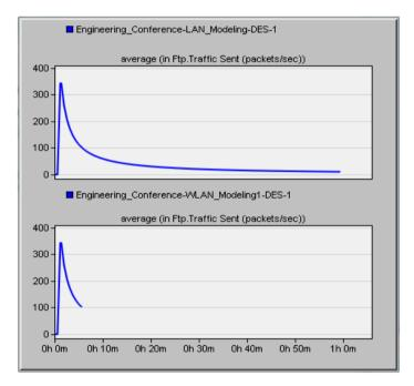
Fig. 4. Comparison of Traffic Sent (packets/sec) in LAN and WLAN Scenarios Displayed in Stacked Statistics
