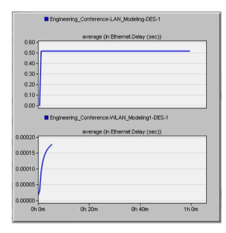
Fig. 3. Comparison of Ethernet Delay (Sec) in LAN and WLAN Scenarios Displayed in Stacked Statistics
