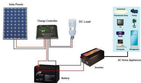
Fig. 2. Typical solar home system components [13].
