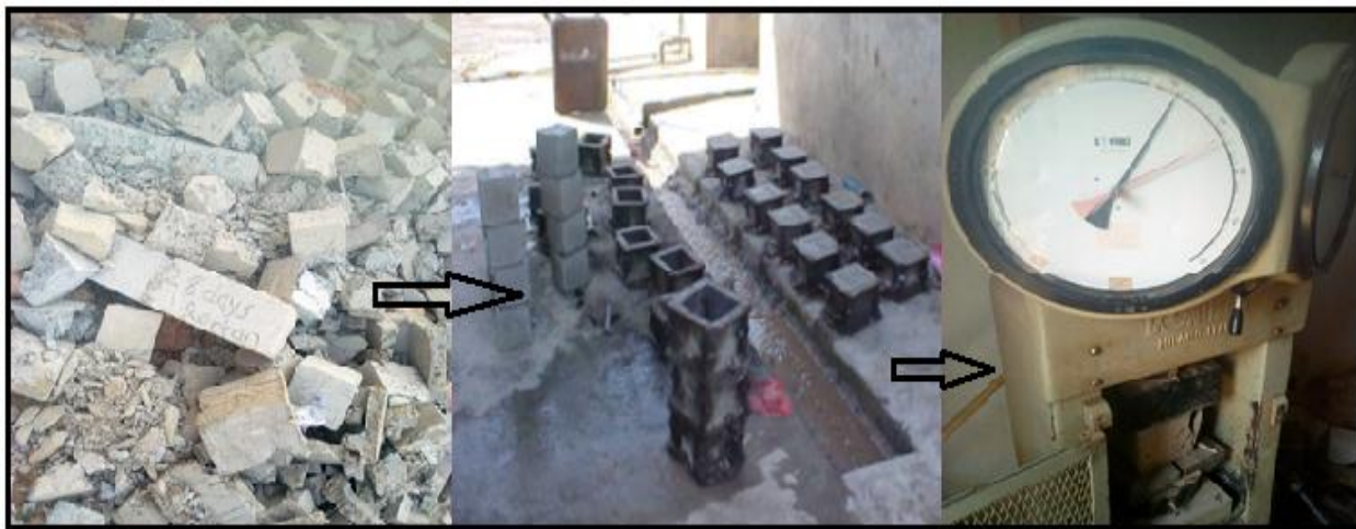
Fig. 1. Pictorial representation of laboratory stages involved in achieving the compressive strength test.
