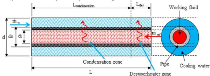
Figure 6: Geometry of the Condenser
