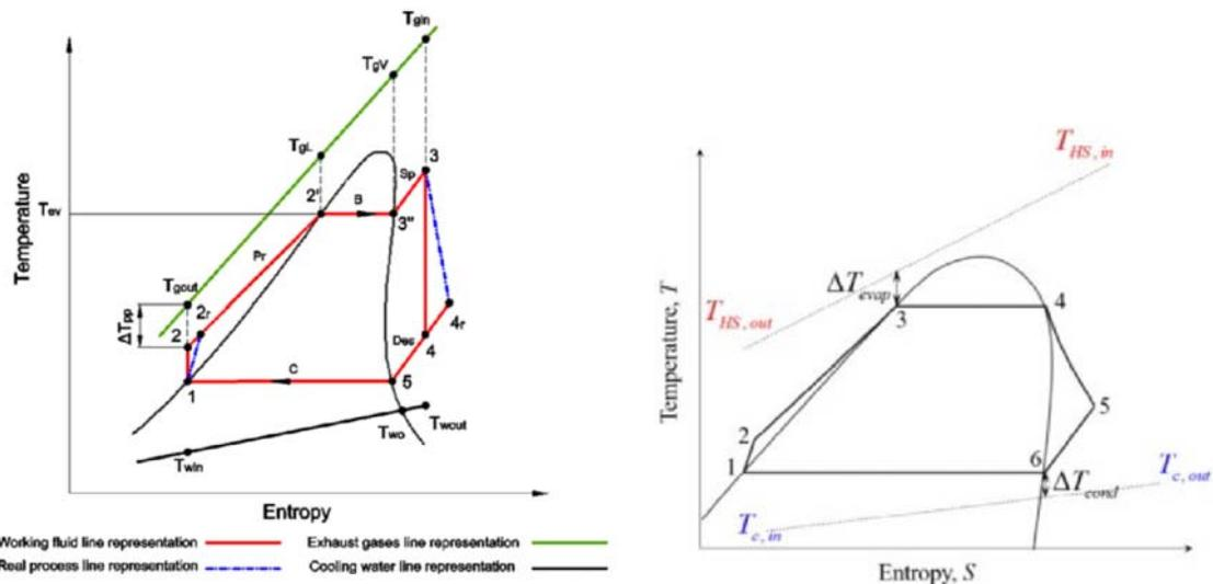
Figure 3: Typical Temperature Profile for (a) subcritical cycle and (b) Supercritical cycle
