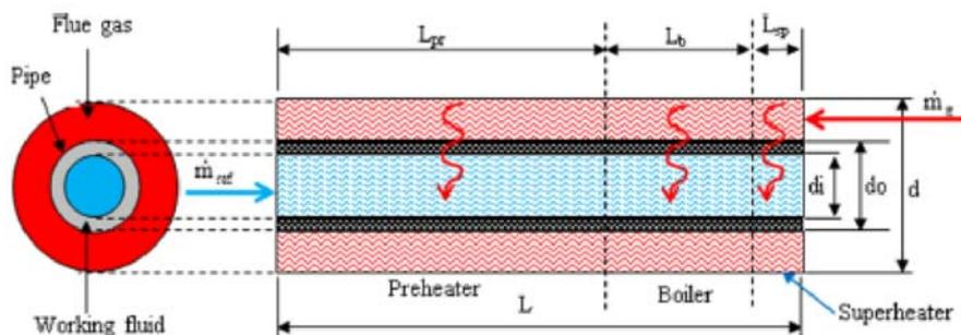
Figure 5: Geometry of the Vapour Generator
