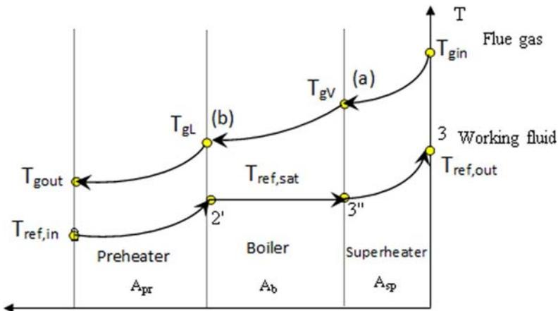
Figure 4: Three zones of the vapour generator (preheater, boiler and superheater)
