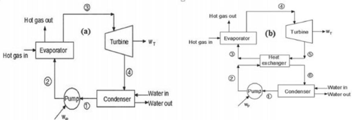
Figure 1: Basic ORC (a) and ORC with internal heat exchanger (b)
